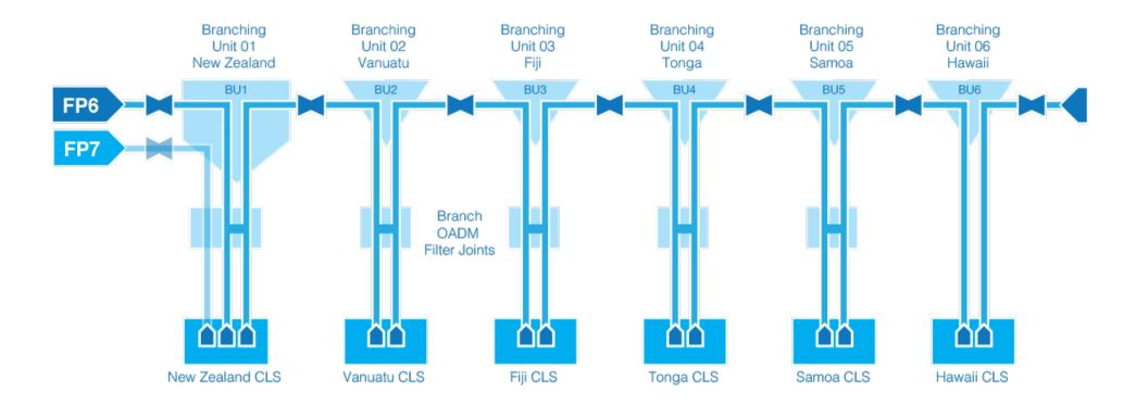
Island Branch OADM filters are set to pass a 1x100Gbs wavelength in each direction towards the terminals. Total drop capacity to each connected Pacific Island is 200Gbs.
