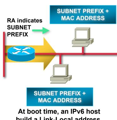
At boot time, an IPv6 host build a Link-Local address, then its global IPv6 address(es) from RA
