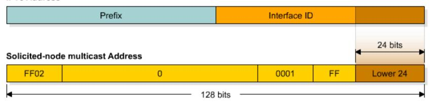
Solicited-node multicast address consists of FF02:0:0:0:1:FF::/104 prefix joined with the lower 24 bits from the unicast or anycast IPv6 address
